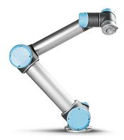
Figure 3: The UR5 manipulator by Universal Robots (seated in Denmark) is a lightweight, adaptable collaborative industrial robot that tackles medium-duty applications.
